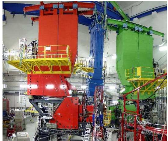
Fig. 4. Photograph of the three high-resolution magnetic spectrometers in the A1 area. Spectrometer A (red) is on the left-hand side, B (blue) in the center, and C (green) is on the right-hand side.
