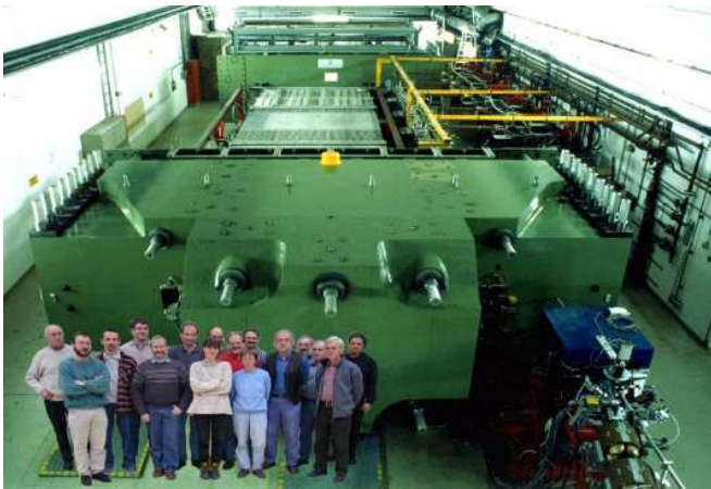
Fig. 2. The MAMI accelerator team standing in front of one of the MAMI B 180° end-magnets. The common accelerating section is located between the magnets on the right-hand side, the separated return paths are on the left-hand side.
