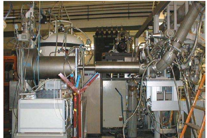
Fig. 7. The Bonn frozen-spin polarized target during a re-polarization cycle. The polarizing magnet is on the left-hand side, the pumping unit on the right-hand side.
